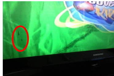
De-lamination: PANEL FAILURE
