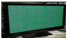
Green lines or a green screen likely caused by a defective main board, LVDS, or T-CON
